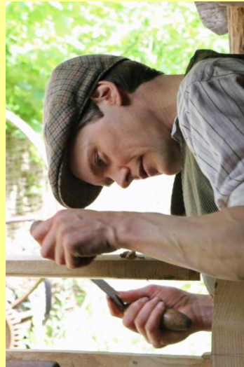
Finishing with a spoke-shave
