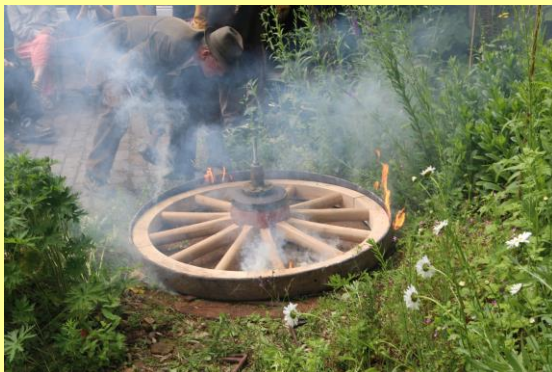
Heating the iron tyre to about 800 0 C
