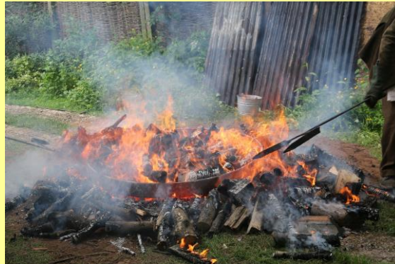
Heating the iron tyre to about 800 0 C
