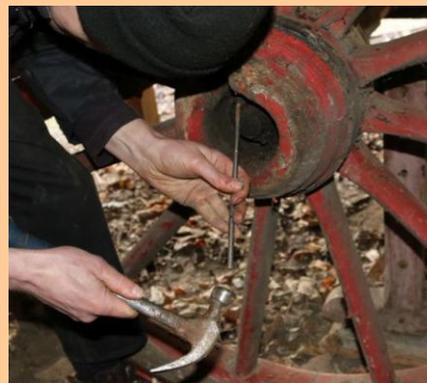
Cut out to allow the pin to be removed
