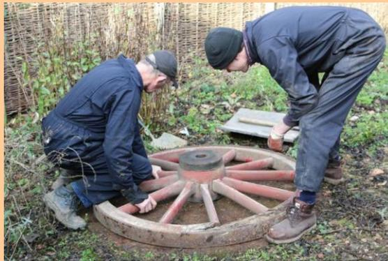
Two wheelwrights from Acton Scott checking the suitability of the tiring platform sited opposite the Drying Shed
